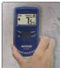
Measure concrete moisture
