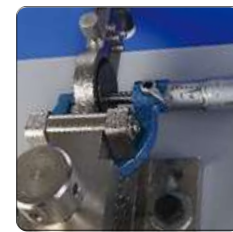
Lapping measuring surfaces of outside micrometer
